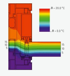
**HIRT kinetics® SF XL:** Highly insulated aluminum profiles with 54 mm insulation stays and a Uf value of 1.418 W/m<sup>2</sup>K. Function glasses up to max 70 mm can be installed.
