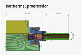
**Best heat insulation:** You save energy with HIRT kinetics® SF 90. Best thermal insulation and the effective air exchange without room cooling are major features. Highly insulated aluminum profiles with 54 mm insulation stays and a Uf value of 1.364 W/m²K. Function glasses up to max 63 mm can be installed. HIRT SF 90 values (examples): Size  $4.50 \times 2.50 \, \text{m}$ , 3-times glass U 0,5 W/m²K: The thermal transfer value of the entire descender front is  $U_W 0.75 \, \text{W/m²K}$ .
